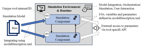
Figure 3: Instantiated Simulation Model and access to its parameters
