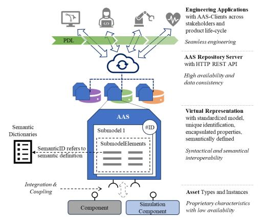
Figure 4: AAS and AAS Repositories for leveraging availability and interoperability of proprietary asset characteristics
