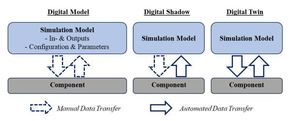
Figure 2: Digital Model, Shadow, Twin, after [3]
