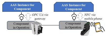
Figure 7: AAS parameter interfaces of the components in operation, left: continuous transfer via OPA UA and gateway, right: intermitted transfer via NFC and mobile app
