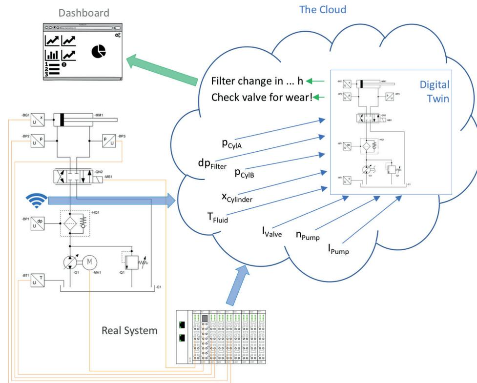
Figure 1: The digital twin as data analyser
