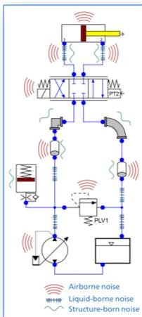
RohrLEX also identified positive displacement pumps as the main source of fluid-borne noise. Due to the discontinuous operating principle of these pumps, the flow discharge delivered to the pipe network consists of a mean, stationary flow with superimposed periodic fluctuations. If the pump is operated with varying rotational speed as is the case with frequency controlled pump drives or vehicle and mobile hydraulic systems, the periodic fluctuations excite the pipe network with
