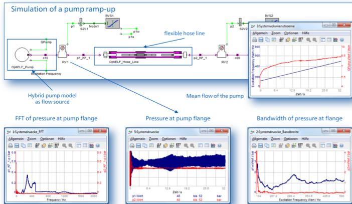
the fact that nonlinearities and certain types of boundary conditions can be taken into account. Due to the modularity of the simulation model, RohrLEx can first analyse the validated components, independently from the original system to which they are attached, and then combine them to a new and optimised system.
