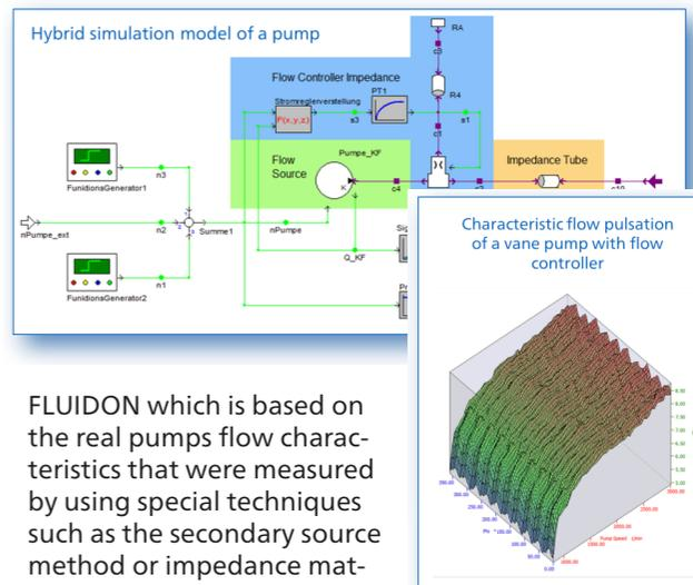
FLUIDON which is based on the real pumps flow characteristics that were measured by using special techniques such as the secondary source method or impedance matching.
