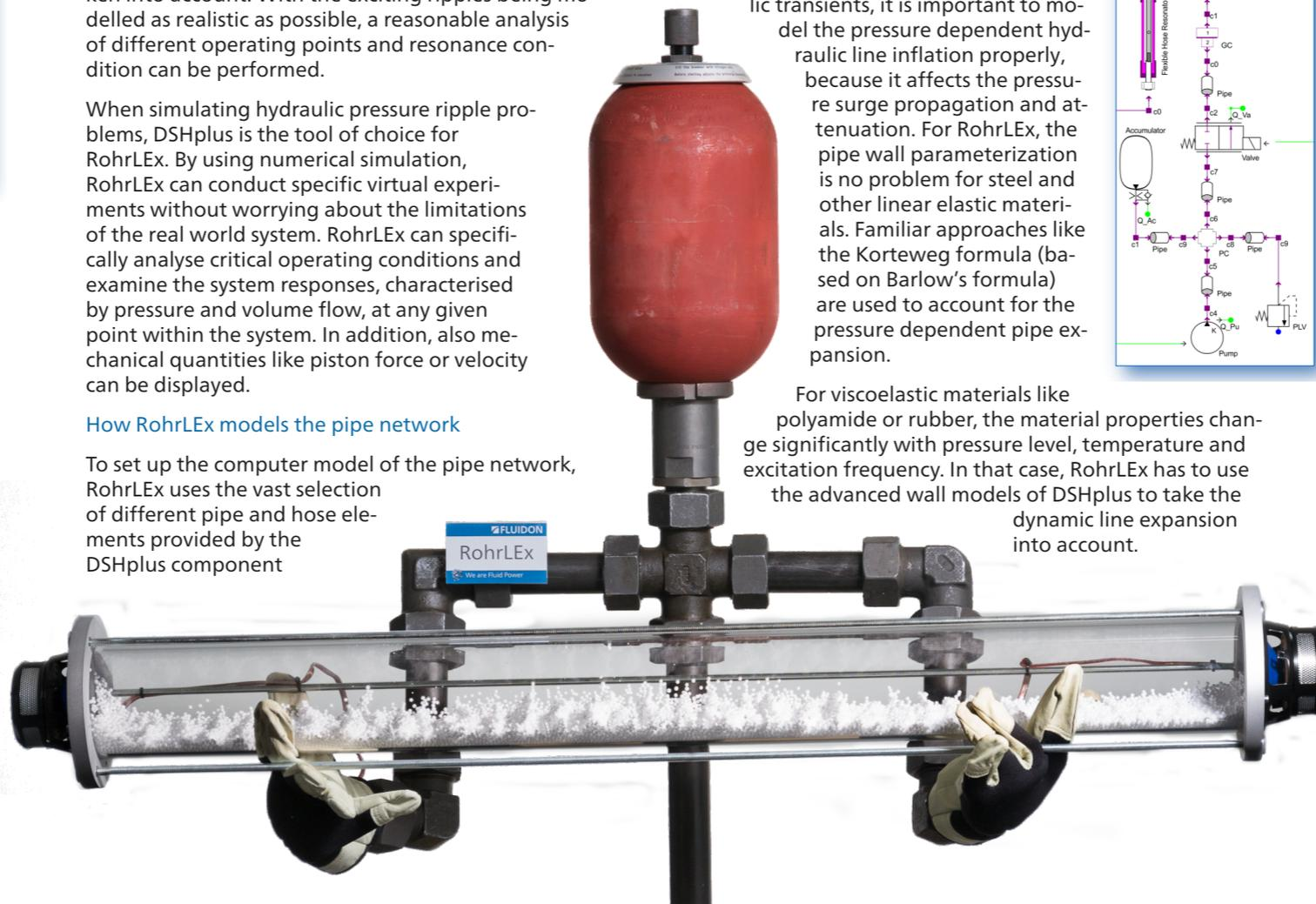
If required, RohrLEX can use the specialised pipe test benches provided by FLUIDON to identify missing material parameters by experiment.
